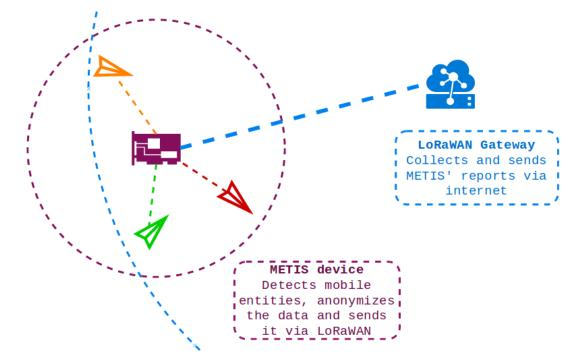
**METIS** is a plug-and-play IoT device. As it comes preconfigured, it only needs a power connection in a location with LoRaWAN coverage.
